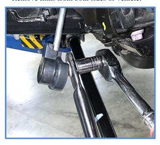
3. King sway bar links are side specific, make sure to install links on the correct side with spacers facing the correct way. Follow the install guide for proper orientation. Failure to install links as shown may cause damage to product and/or vehicle.
