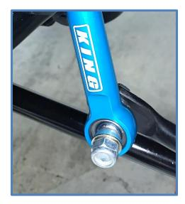
6. <u>Right Side</u> - Place the supplied 12mm bolt with washer through the sway bar link and into the upper mount — on the frame with the longer spacer facing the mount. Place a washer and nut on the bolt and thread nut on by hand for now to hold in place, you will torque all bolts when both links are installed.
