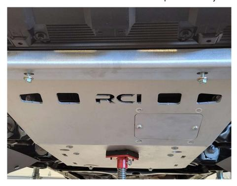
b. 2 sets of M8 hardware secure the center of the skid plate assembly.
