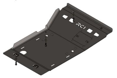
a. 2 sets of M8 hardware secure the front of the skid plate assembly.
