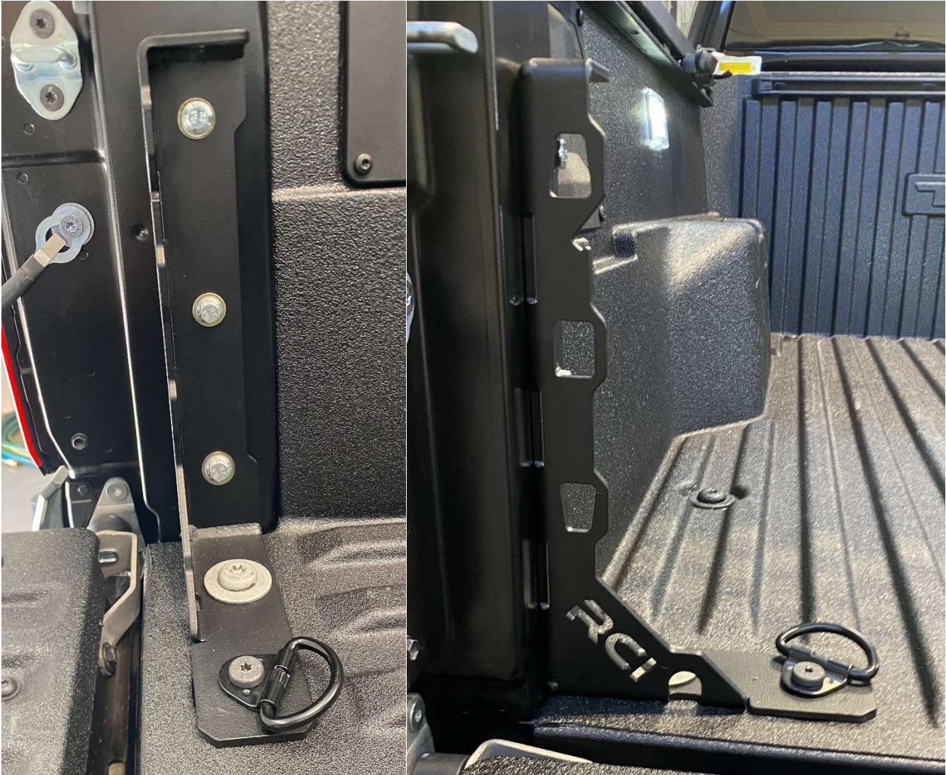
Figure 10: Correct installation of bed stiffener.
