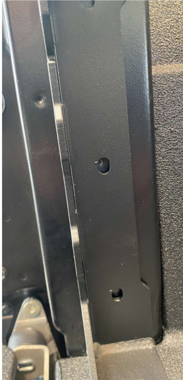
Figure 4: Example of marking hole locations.
