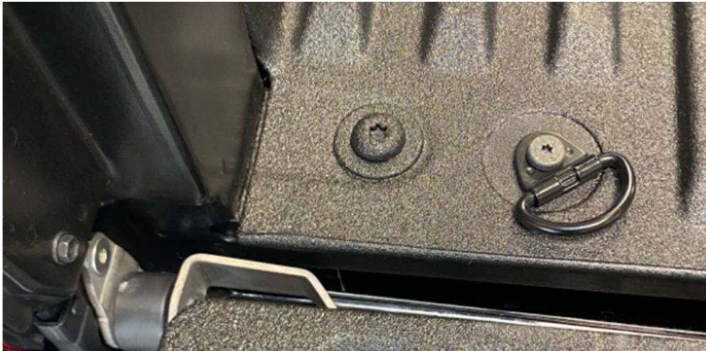
Figure 2: OEM bolts to remove.
