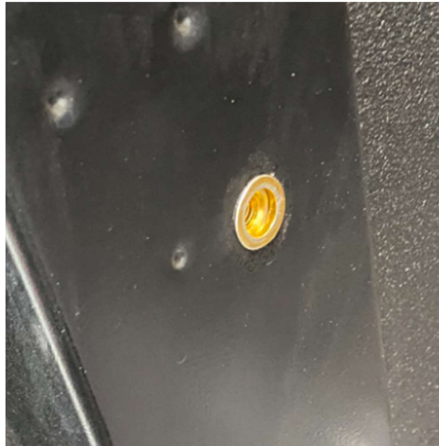
Figure 9: Correct rivet nut installation.
