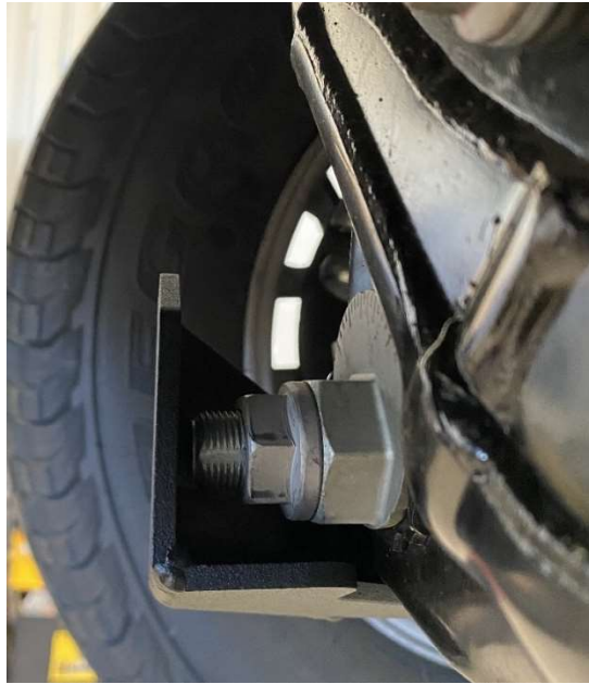
Figure 4: Example of correct gap between alignment bolt and skid.
