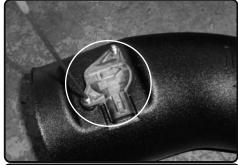
**9.** Install the MAF sensor into the intake tube, secure using provided M4 button head screws.
