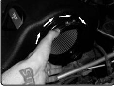
**21.** Once seated, rotate in either direction 1/4 turn till filter locks.
