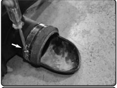
**15.** Secure the inlet scoop with the provided #56 band clamp.
