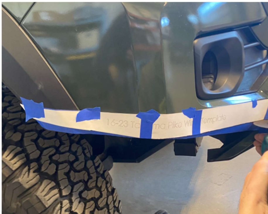
Figure 3: Template correctly installed on bumper.
