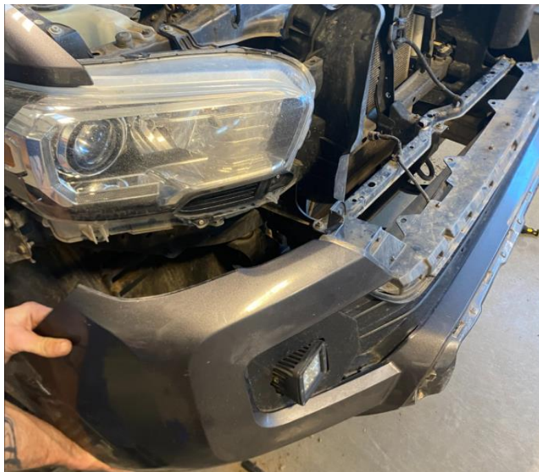
Figure 9: Example of the bumper half removed.
