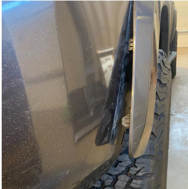
Figure 8: Lower fender pulled away.
