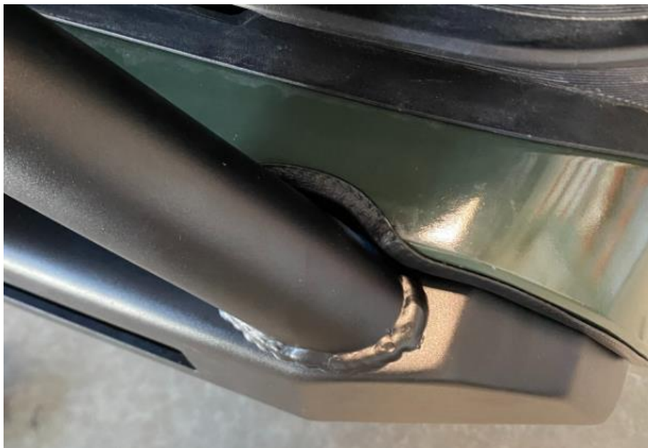
Figure 21: Example of finished cut for hoop.
