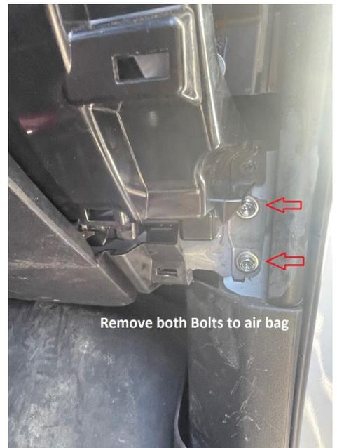
**Step 4: Remove all screws holding in the glove box,
