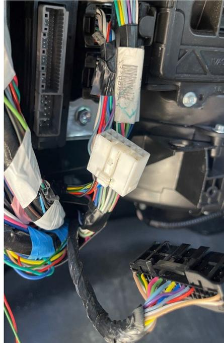
Step 6: Install the 40 pin and 10 pin jumper Harnesses into the 4x4 module and connect to the main wiring harness as shown in pictures below. Then secure any loose wires.
