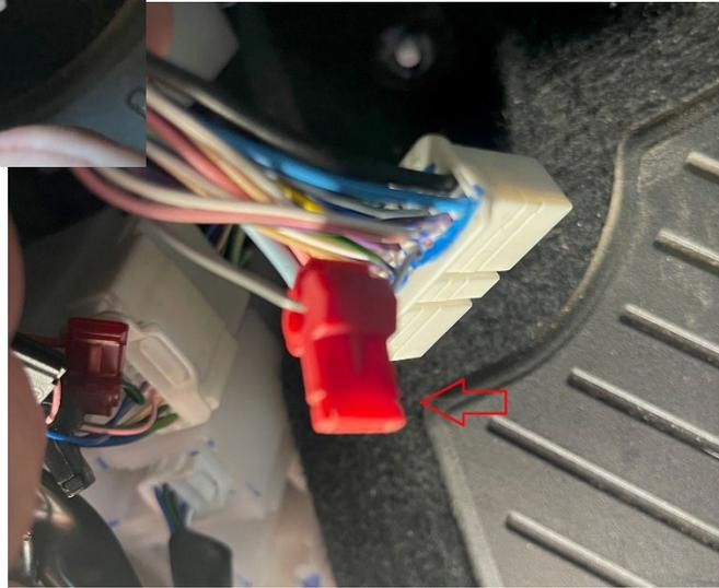
Step 11: Connect the AnyTime Locker's Gray/white wire with provided spade connector to the T-Tap and tie up and loose wires.
