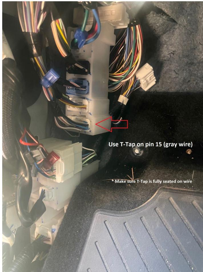
Step 10: connect the T-Tap to the Gary wire on connector IA5.
