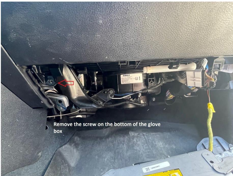
Step 5: Locate the 4x4 module and unplug the 40 pin and 10 pin connectors.
