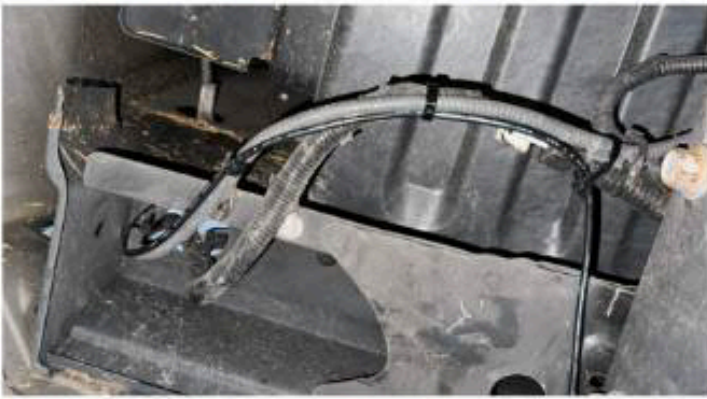
25. Perform the same steps on the opposite side of the truck. The long Y adapter end should be zip tied to factory loom under the bumper area.
