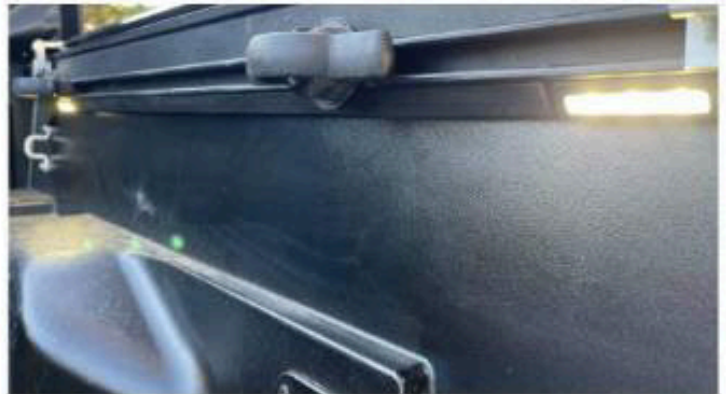
30. Test functionality. When the Cargo Switch inside the truck is in DOOR position dropping the tailgate should turn all of the lights on. Re-assemble truck. INSTALL COMPLETE.
