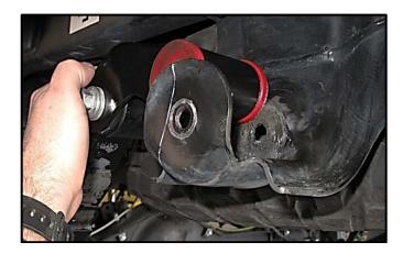
17) Lower the axle onto the spring perches.
