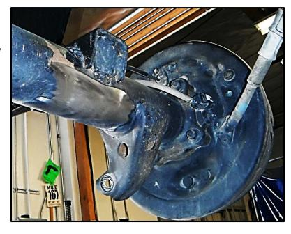
One spring at a time, use a jack under the center pin and jack up the spring until the shackle is above the rear shackle mount, then pull the leaf spring down until the shackle hole lines up with the frame mount hole and install the bolt. (Repeat on other side, this is easiest with two people)
