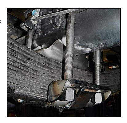
18) Drill out the stock emergency brake cable mounts to a 3/8" hole. Install onto new leaf springs (the spring clamp bolts are 3/8").
