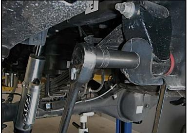
10) Remove the front spring hanger bolts. Now remove the leaf springs.
