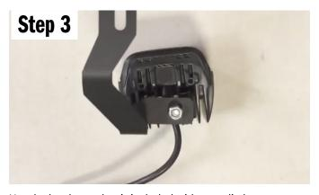
Use the hardware that is included with your ditch mounts to connect the pod to the mount. Do NOT use the hardware included with your pods. Put the bolt through the u-bracket, then through the ditch mount, then install your lock nut on the bottom. Tighten so it doesn't flop around, but leave loose enough to make light adjustments after mounting to your vehicle.
