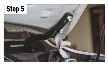
Remove the nut/bolt and move the mount in place, then put the nut/bolt back in place, snug but not tight.
