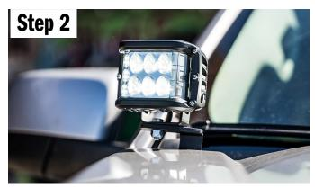
Install your pod to your ditch mount in the correct direction. If you have side shooter style pods, make sure you have the correct pod on the correct bracket. For example, make sure the passenger side pod is on the passenger side bracket. For side shooters, make sure the side LEDs are pointing away from your hood.
