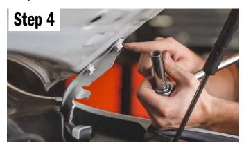
Now we are going to install the bracket to your vehicle. Start by loosening the top nut or bolt that holds your hood in place.
