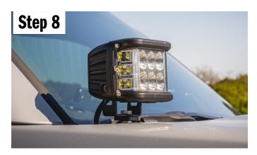
Tighten all the bolts and close your hood. Check for clearance and make any necessary adjustments if needed. Lastly you want to aim your lights to the desired spot, then tighten the pod the u-bracket, and u-bracket to the ditch mount.
