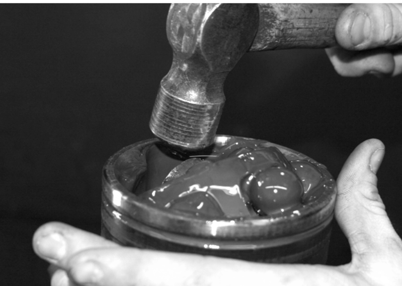
9. Tap the remnant of the axle with a hammer to rotate the CV far enough to remove one ball at a time. Use a pick or small screwdriver to help.
