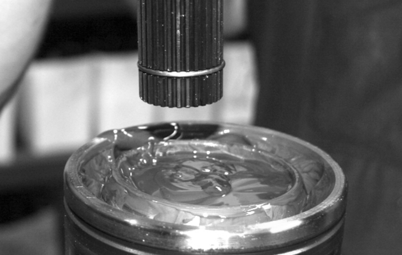
18. The new axle shaft has a new retaining ring that expands once it goes through the star. Align the splines and push the axle so the retaining ring is compressed inside the star. Use a rubber mallet to tap the axle through the star. Make sure it is seated all the way down.
