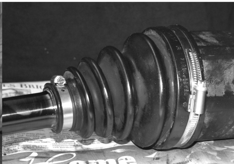
23. Attach the inner CV boot and tighten the boot clamps.
