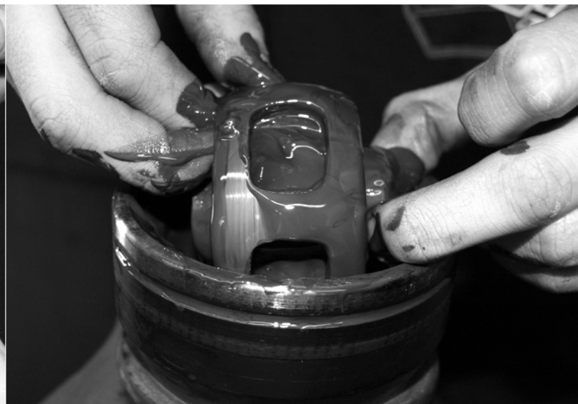
10. Once all the balls are removed, rotate the CV star and cage so they are straight up and down.
