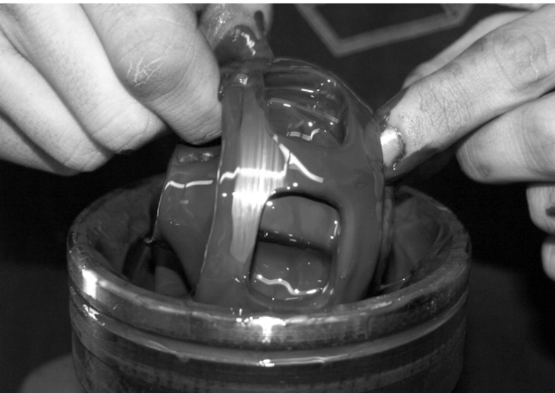
11. Rotate the CV cage windows so they align with the grooves and pull internals out from the CV joint. Take note of which side of parts faces up towards axle so they are reassembled exactly the same.
