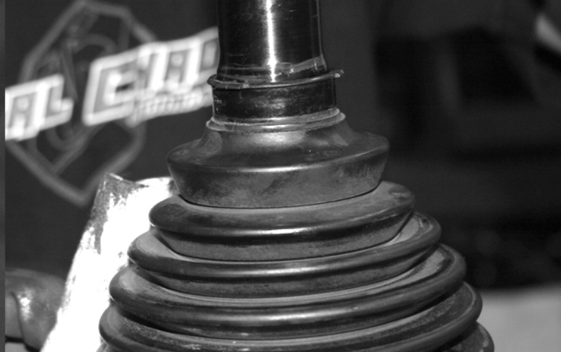
19. Slide the factory outer boot onto the opposite side of the axle and attach it to the CV joint. Use new CV boot clamps.
