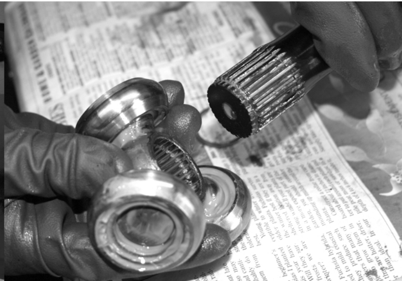
21. Mate the inner CV star with the axle and install the snap ring.
