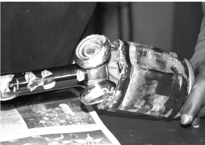
22. Slide the inner CV housing onto the axle.
