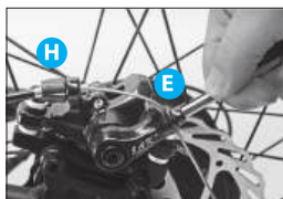
(fig.2) When pulling the cable through for re-tightening make sure NOT to raise the Caliper Arm as this will reduce effective braking
