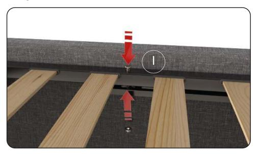
a.On each side of the side rail, mount the base to the lift up arms, using the 54mm Allen key bolts x 3 each side.
