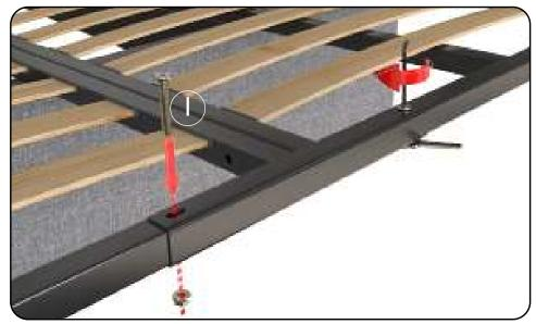
Secure the U channel, by using the 54mm Allen Bolt, with Flange Nuts. By using the Allen key and 12mm spanner.
