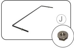
Fit on each side a Flange Nut, this can be positioned to suit the height of your mattress.
