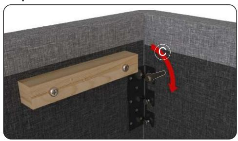
Tighten all bolts with 13mm spanner (C)
