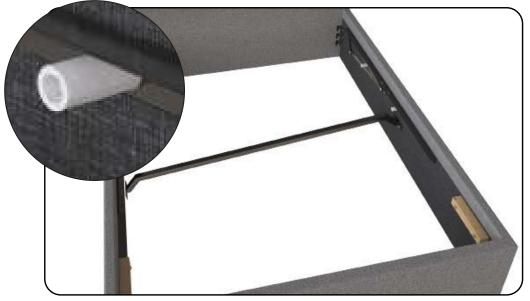
a. Insert the cross bar into the middle of the bed, where the insert nuts are positioned.
