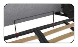
Now slot this into the holes at the centre of the ottoman base. Please ensure the base is positioned correctly, i.e. the mattress stopper should be at the headboard position.
