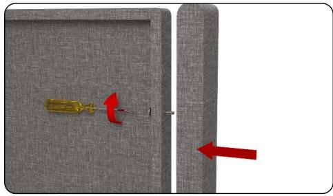
If your ottoman bed has wings mounted to the headboard, please fit these now. Use the M8 100mm pozi bolt x 3 each side to secure the wings to the headboard.
