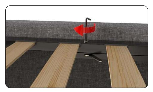
b.Once the bolts are slotted in position, on the bottom side secure by using a flange nut. At this stage leave the bolts slightly loose, until you have all 6 bolts in position.
