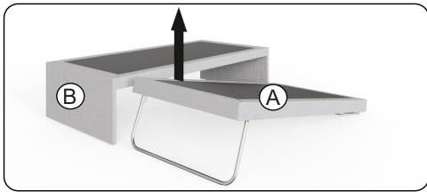
Lift up one end of frame (A) and the leg will automatically drop down.
