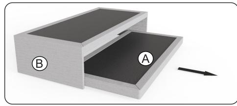
To use frame (A), slide it out from under frame (B)
