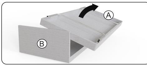
Turn frame (A) over so it is the correct way up. (*This is a two man lift*)
