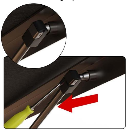
Using a flathead screwdriver, push outer lever upwards and pull the strut from the fitting.
