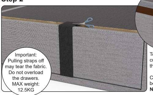
To release drawers; carefully cut restraining straps and trim the excess.
