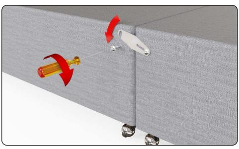
Use 2x bolt (B) to fit each base connector (A)
