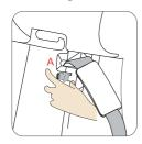
Loosen the cloth cover inside the seat and adjust the headrest to the highest position (see page 5, 3.2 of the manual). Remove the chest strap from the hook and pull out the chest pad. Repeat for the other side.
