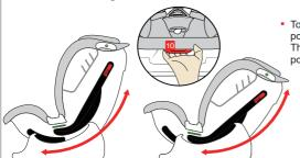
To recline the seat pull the recline adjuster and position the seat to your required recline angle.
