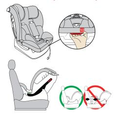
Method: Pull the recline adjuster 10 under the seat, adjust to the most reclined position.
