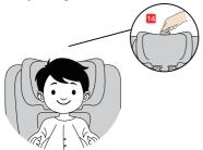
As shown in the picture, you can adjust the headrest up and down by pulling on the headrest adjuster and adjust the headrest to a position suitable for the child's head
