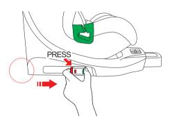
STEP 1: Ensure that the support leg is concealed and adjust the seat tilt angle to the first gear. Position the seat against the car seat.
