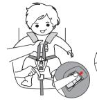
To loosen the shoulder harness, simultaneously press the adjuster button located beneath the cover and pull both shoulder straps forward.
