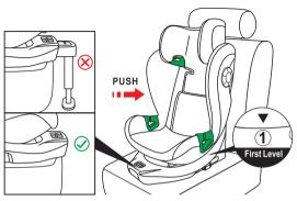
STEP 2: Place the child in the seat and secure them by following the path 123. Ensure that the seat belt is tightened adequately.
