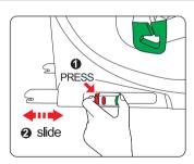
To retract or unlock the ISOFIX interface. press and hold the switch in place.
