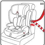
**Step 3:**Pull out the diagonal belt together with lap belt and pass them through the belt route slot of backrest(D3).
