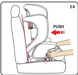
**Step 4:** Check to ensure that the Ezfix locking system turns to green and make sure child seat is firmly connected(E4).
