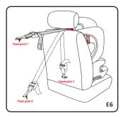
**Step 6:** Connect top tether with the fixing point on the car(E6).
