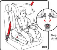
**Step 2:**Release the buckle, and put the child into the safety car seat(D10).
