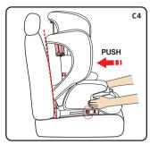
**Step 4:** Ensure that the Ezfix turns to green and make sure child seat is firmly connected(C4).
