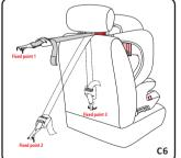
**Step 6:** Connect top tether with the fixing point on the car(C6).
