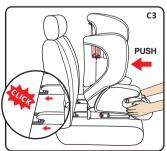
**Step 3:** Push the child seat in the direction illustrated and insert the Ezfix connectors into the Ezfix guides (C3)
