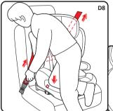
**Step 6:**Pull the car seat belt following the direction of the red arrow to ensure that the belt is tight (D8).
