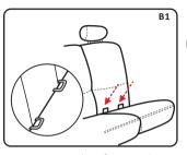
**Step 1:**Locate the Ezfix connection points in the car.
