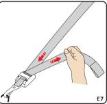
Step 7: Pull the belt of top tether until the adjuster shows green(E7).
