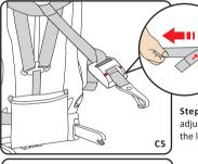
**Step 5:** Locate the top tether and press the adjusting button. Adjust the top tether belt to the longest it can go (C5).
