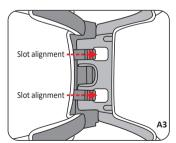
**Step 3:** Place the backrest hooks inside the base securely.
