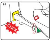
**Step 3:** Push the child seat in the direction above (B3) and insert the Ezfix connectors into the Ezfix guides (B3, B4). Check that the Ezfix locking system turns green to ensure that it is locked and make sure that the child seat is firmly connected (B4).
