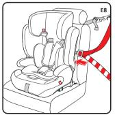
**Step 8:**Pull out the diagonal belt together with lap belt and pass them through the belt route slot of backrest (E8).
