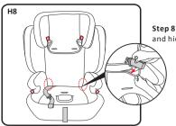
Step 8:Fold the strap of both sides and hide under the booster cover
