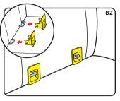
**Step 2**: Insert the Ezfix guides into the Ezfix connection points.
