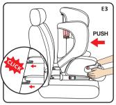
**Step 3:** Push child seat following the direction illustrated, until the Ezfix connectors are completely locked with the connection points of the vehicle (E3)
