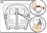
**Step 5:**Pull out the harness from the slot under the safety car seat.
