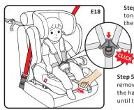
Step 4. Align the left and right buckle tongues to one tongue and insert into the buckle until you hear a "Click"(E18).
