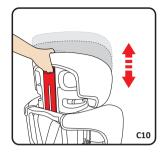
**Step 3:**Pull the height adjuster to adjust the height of the harness and the headrest according to the child's height(C10).
