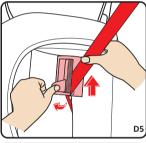
**Step 5:** Clip the diagonal belt into the locking clip.(D5,D6,D7).
