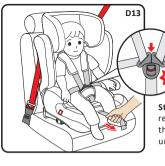
Step 4. Align the left and right buckle tongues to one tongue and insert into the buckle until you hear a "Click" (D13).
