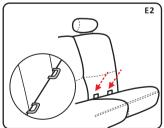
**Step 2:**Locate the Ezfix connection points in the vehicle.
