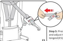
**Step 5:** Press the adjusting button and adjust the belt of top tether to the longest(E5).
