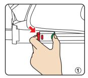
Press the red button to release the Ezfix connector and take away the seat
