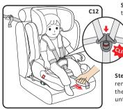
Step 4. Align the left and right buckle tongues so that they form one tongue and insert into the buckle until you hear a "Click" (C12).
