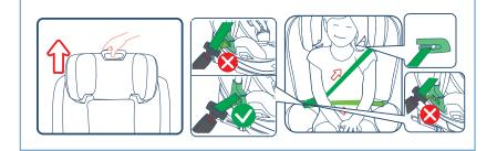
Adjust the height of the headrest to suit your child. Put the vehicle belt through the belt guide. Place your child into the baby car seat and let the vehicle belt pass the belt guide. Fasten the vehicle belt with an audible sound"click".
