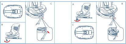
First, remove the supporting leg from the bottom of the seat. When the supporting leg is rotated outward to 45°, the supporting leg assembly can be pulled out outward.
