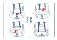
Find the metal plate of buckle latches under the memory foam, guide the metal plate through the slot and grasp it from the hole underneath the seat base to remove one side of harness strap; Repeat this step to remove the another side of harness strap.
