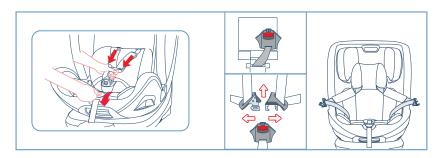
Loosen the shoulder straps by pressing the harness adjusting button and pull the harness shoulder as far forward as possible.
