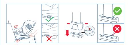
Grasp the seat body to check the seat if it is fastened tightly or shakes, meanwhile observe the ISOFIX red/green indicator. If the seat shakes and the ISOFIX connectors are pulled out, please repeat the above steps and install it again.
