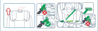
Adjust the height of the headrest to suit your child. Put the vehicle belt through the belt guide. Place your child into the baby car seat and let the vehicle belt pass the belt guide. Fasten the vehicle belt with an audible sound"click".
