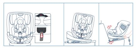
Tighten the harness adjusting strap and make sure the harness is reasonably tight. It should restrain but not make the child uncomfortable.
