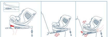
Unfold support leg until it locks in place. Press the ISOFIX release button to slide the ISOFIX connectors to the end.
