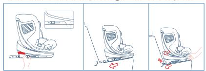
Unfold the support leg until it hides in place. Press the ISOFIX release button to slide the ISOFIx connectors to the end.
