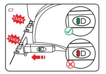
Step 6: Ensure that the EZFix locking system turns green to confirm that the child seat is firmly connected.
