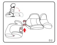
Step 2:Separate the backrest from the booster by unhooking the two parts.see D2
