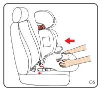
Step 5: Place the child car seat on the vehicle seat and push back in the direction of the EZFix guides. Insert the EZFix connectors into the guides.
