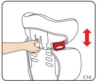
Step 9: Adjust the height of headrest and belt slot to a suitable height for the child.(C10,C11)
