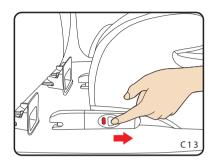
Step 11: To release the child car seat pull on the locking mechanism.when you hear a "Click" and the indicator turns red and the EZFix connector has been released. Then pull your child car seat forward.
