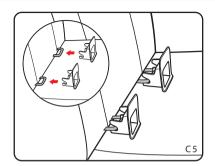
Step 4: Insert EZFix guide into EZFix connection
