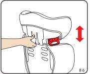
Step 5: Adjust the height of headrest and belt slot to suitable height of child (B6, B7)
