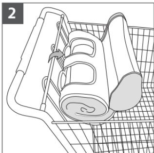
3. Remove the cover's hood from the backrest, then flip it over the rolled cover.
