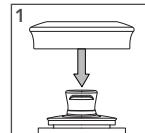
**Note:** Hold the base to unscrew the collar from the cup.
