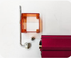
Remove the protective cover, air guide cover, nozzle, and window mirror.
