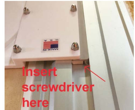
Figure 3 Place over track, Loosen all three screws. Squeeze and then tighten.
