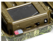
② Install micro SD card
