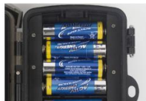
① Install Batteries
