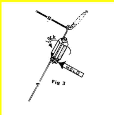
3) Turn Kwik Twist over and insert wire in slot along side of Kwik Twist tool. Lock wire into position by holding knurled end with one hand and turn hex with other hand as illustrated in Fig. 3.
