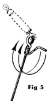
5) Remove from tool by unlocking tool opposite direction of Fig. 3. To break off wire clean, shape wire into "L", Fig. 5. Using "L" shaped handle to hold wire, rotate close to main shaft of leader and wire will snap off clean.
