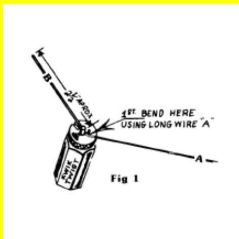
1) Place wire on top of knurled end of Kwik Twist between pins. Extend "B" section of wire about 2 1/2" as illustrated in Fig. 1. This centers the eye of the leader you are now making.
