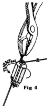
4) Turn tool approx. 4 to 6 turns while holding eye with pliers or tool provided in kit. Holding eye of leader with pliers is the best way when learning to make your own barrel wrap leaders. Illustrated in Fig. 4.
