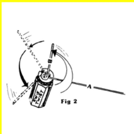
2) Now take "B" and start forming the eye of the leader by turning the wire around the center pin. Be sure to pass over the top of the small pin to complete this bond. Illustrated in Fig. 2. remove wire from tool. Now put snap or swivel on loop.
