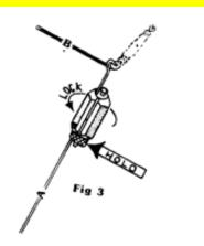
3) Turn Kwik Twist over and insert wire in slot along side of Kwik Twist tool. Lock wire into position by holding knurled end with one hand and turn hex with other hand as illustrated in Fig. 3.
