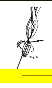
4) Turn tool approx. 4 to 6 turns while holding eye with pliers or tool provided in kit. Holding eye of leader with pliers is the best way when learning to make your own barrel wrap leaders. Illustrated in Fig. 4.
