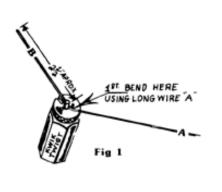
1) Place wire on top of knurled end of Kwik Twist between pins. Extend "B" section of wire about 2 1/2" as illustrated in Fig. 1. This centers the eye of the leader you are now making.
