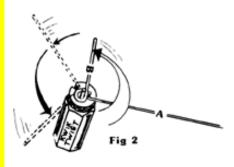
2) Now take "B" and start forming the eye of the leader by turning the wire around the center pin. Be sure to pass over the top of the small pin to complete this bond. Illustrated in Fig. 2. remove wire from tool. Now put snap or swivel on loop.
