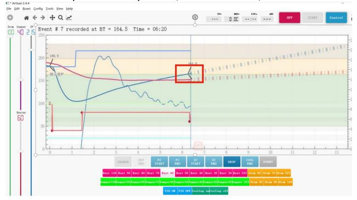
12.When First Crack, Click "FC START", "Heater 20", "Damper 80"
