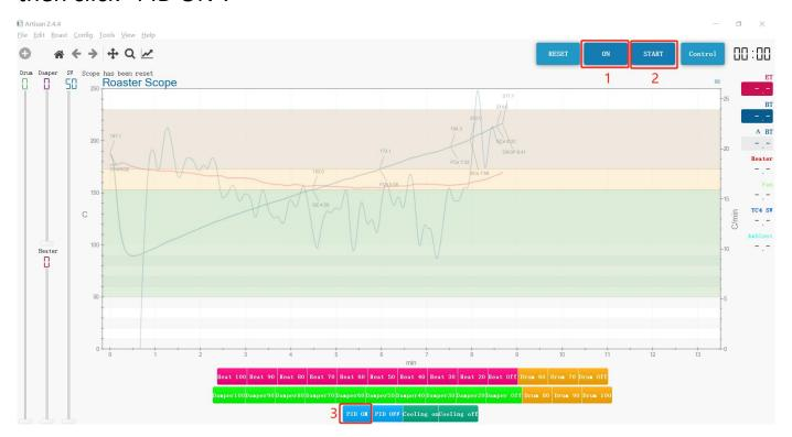
4. Parallel lines will appear when the roaster reaches the preset temperature of the background roasting curve. It's time to pour in green beans when temperature reach the presetting value of the background roasting curves.
