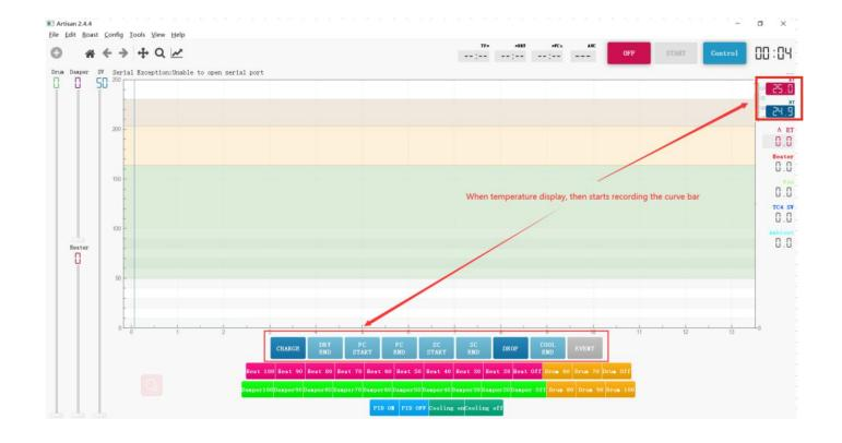
8. Click "Drum100RPM", "Heat 100", Drag the "SV" value to  $180\,^\circ\text{C}$  (setting max drum temperature).Then the roaster will preheat to  $180\,^\circ\text{C}$  automatically.
