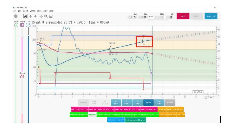
13. When first crack finish, click "Heater off, Damper off", then click "DROP". (Turn on the cooling fan while automatically turning off the heat)
