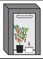
The  $CO_2$  Generator is designed to operate in sealed grow room spaces such as greenhouses or horticultural tents. A 5L Generator can supply enough  $CO_2$  for up to 1.2m x 1.2m. / 4ft x 4ft A 10L Generator can supply enough  $CO_2$  for up to 2.4m x 2.4m. / 8ft x 8ft
