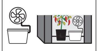
Always position your  $CO_2$  Generator on the floor, never raise it. If you have a fan or air circulation system route the upper pipe of the Generator into the back of a circulation fan so  $CO_2$  is distributed evenly throughout the growing environment.
