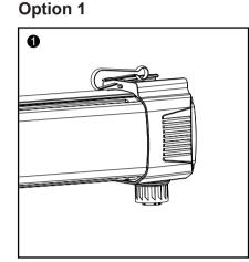
1. Put the hooks into the holes on both sides of the light bar
