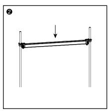
Step 2: To install the light bars, align the holes on both sides of the ICL-300 light bar with the vertical tubes. Align the mounting bracket on the vertical tube, with the bracket on the ICL-300 to ensure a secure connection between the light bar and the vertical tubes. It is essential to conduct a thorough inspection to ensure proper alignment and secure installation before proceeding.
