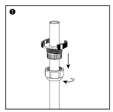
Step 1: Utilize the two Collar Mounts which are provided with each ICL-300 to securely fasten the ICL-300 onto two PVC or metal pipes or conduits with a diameter ranging from ¾" to 1" or 18mm to 25mm. Begin by loosening the screw cap on the adjustment knob, allowing the tubes to pass through the screw cap. Next you can position both ends of the ICL-300 to the desired orientation / height and secure it in place by tightening the screw cap.
