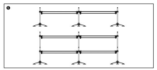
Step 5: To validate the stability of the installation, double-check that all of the screw-nuts have been tightened and all of the ICL-300 brackets are aligned and joined to the TSD-1 correctly. Then gently push and shake the stand. If the stand remains steady without any notable movement, the installation can be considered successful and complete. Make adjustments or tighten hardware if the assembly seems loose or unstable.
