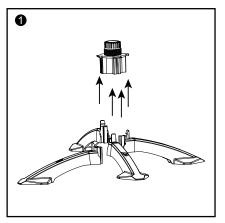
Step 1: Begin by inserting each of the 4 molded legs into the central mounting bracket. Ensure that all 4 legs are securely installed and have "snapped" into place.
