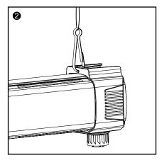
Step 2: The ICL-300 can be suspended from the ceiling or from above using an appropriate length of rope, wire rope or cable. Select a secure mounting point using appropriate hanging hardware. Exercise caution during this process to ensure that the ICL-300 is correctly positioned and securely fastened.
