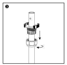
Step 3: Utilize the two Collar Mounts which are provided with each ICL-300 to securely fasten the ICL-300 onto the aluminum tubing. Begin by loosening the screw cap on the adjustment knob, allowing the tubes to pass through the screw cap. Next you can position both ends of the ICL-300 to the desired orientation / height and secure it in place by tightening the screw cap.
