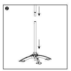
Step 2: Loosen the screw cap to create an opening, allowing the aluminum tube to pass through the screw cap at the top of the central mounting bracket. Make necessary adjustments and firmly tighten the screw cap. Users have the option to utilize one or two sections of aluminum tubes.
