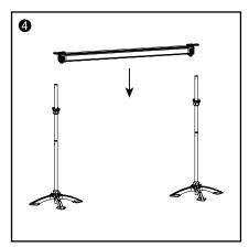
Step 4: To install the light bars, align the holes on both sides of the ICL-300 light bar with the aluminum tubes. Align the mounting bracket on the tube, with the bracket on the ICL-300 to ensure a secure connection between the light bar and the tubes. It is essential to conduct a thorough inspection to ensure proper alignment and secure installation before proceeding.
