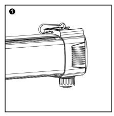
Step 1: Carefully insert the hooks into the two mounting holes located on the opposing sides of the light bar. Ensure that the hooks are firmly secured in place, providing a secure connection for the subsequent steps.
