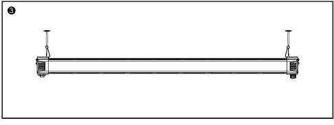
Step 3: Once the ICL-300 has been installed and is hanging freely, test the support mechanism to ensure it is capable of supporting the full weight of the ICL-300.
