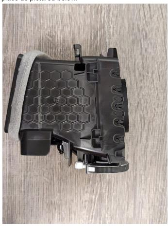
c. Ensure that the two tabs on the right side insert have snapped firmly into place as pictured below.
