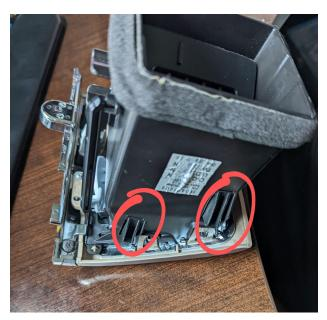
d. You should now have the HVAC vent assembly fully removed from the vehicle so that you may disassemble it and install your PazPodz insert.
