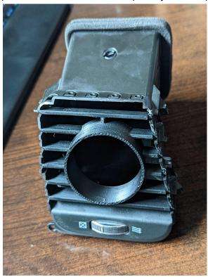
b. Ensure that all of the pins on the insert have snapped firmly into place on both sides of the vent as pictured below.
