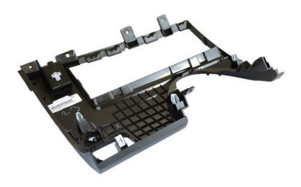
d. CAUTION: You do not need to remove this trim completely. In fact, there are additional steps necessary to remove the airbag module and retaining clips at the bottom of this trim panel if you wish to remove it completely.
