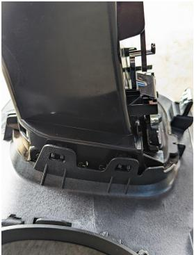
c. You should now have the factory vent duct assembly fully removed like below.
