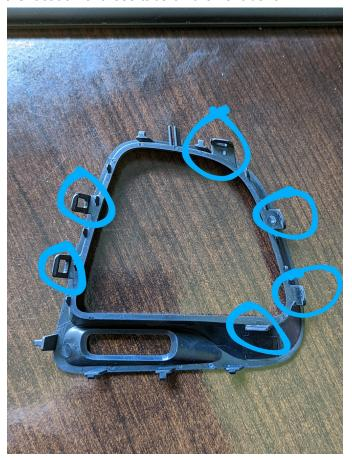
c. Next, remove the vent duct from the instrument cluster bezel by gently prying the large retaining clips. There are two on each side.
