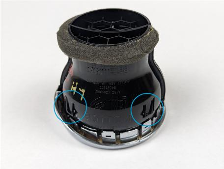
d. You should now have the factory vent duct assembly removed from the dashboard instrument panel trim bezel.
