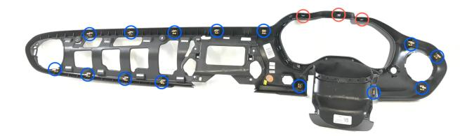
c. Some of the metal clips from the tabs may remain in the dash after removing the bezel. Carefully remove them from the dash and place them onto the plastic tabs that are part of the bezel to make reinstalling the bezel easier in the later steps.
