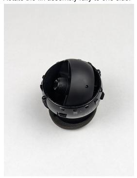
c. Slowly and firmly pull the fin assembly out from the front of the vent. The vent duct will likely flex to allow the fin assembly to pop out. If the vent duct separates along the seams, this is okay as the chrome trim ring and tab connection points on the dash panel will push the two halves back together when reinstalled.
