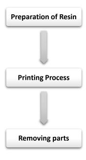
The material should be processed at room temperature. Before usage the material should be shaken well. Pour it slowly in the vat and wait a couple minutes, until smooth, bubble-free surface is obtained before starting the print job.
