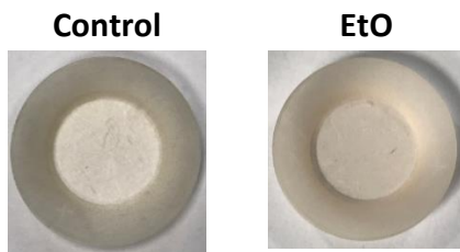
Figure 4 Color discs before and after EtO sterilization
