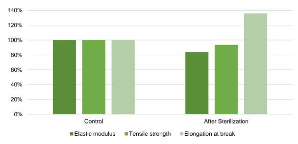
Figure 5 Tensile properties comparison of the EtO-treated samples
