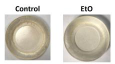
Figure 4 Color discs before and after EtO sterilization
