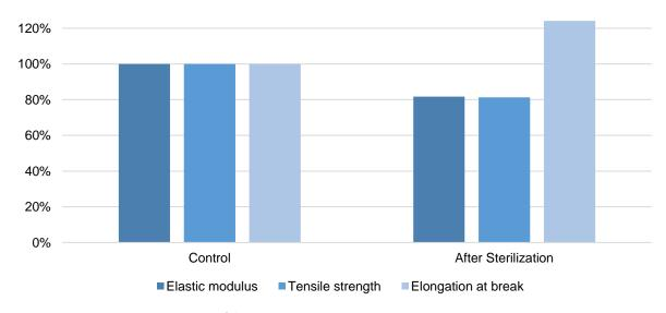
Figure 7 Tensile properties comparison of the Steam-treated samples
