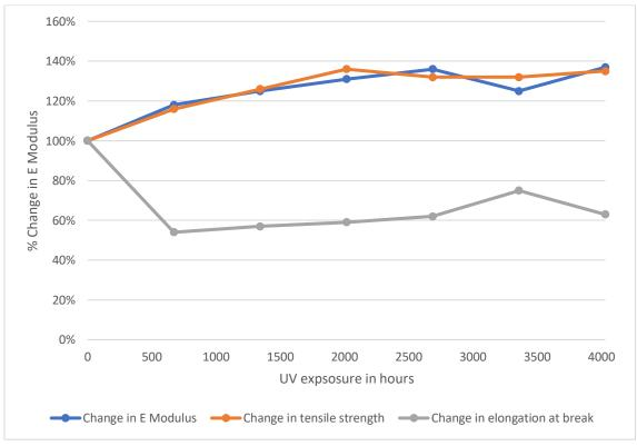
Figure 2 Change in mechanical properties over the course of 4032 hours of UV exposure
