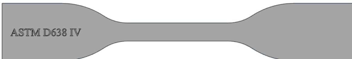
Figure 1 Tensile bar ASTM D638 IV
