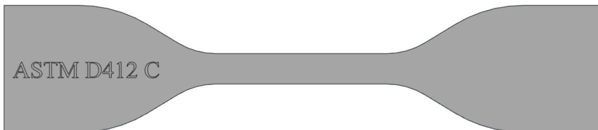
Figure 1 Tensile bar ASTM D412 Type C
