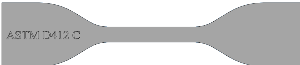
Figure 1 Tensile bar ASTM D412 Type C
