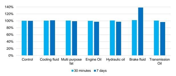
Figure 4 Change in weight in chemical fluid
