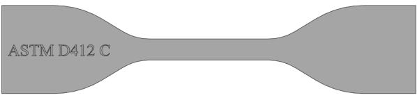
Figure 1 Tensile bar ASTM D412 Type C
