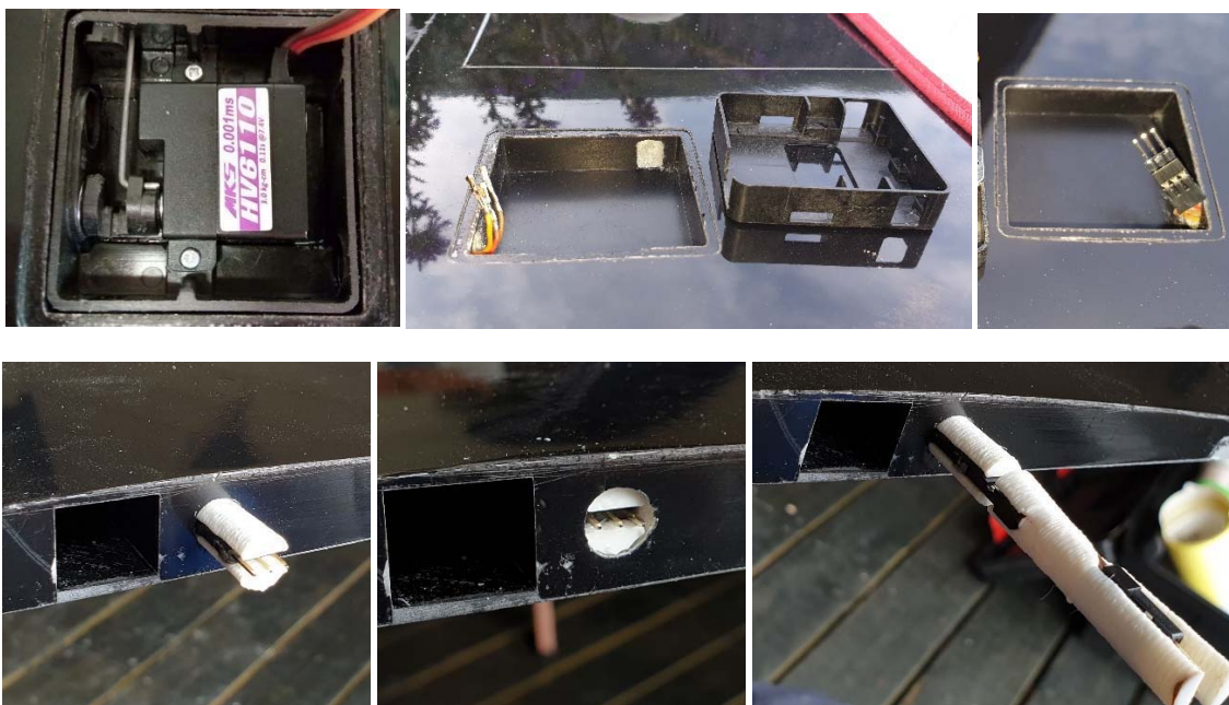
Aileron and flap servo details – below: Contact holder arrangement glued in
