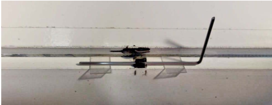
Distance aileron to pin is 0,5mm
