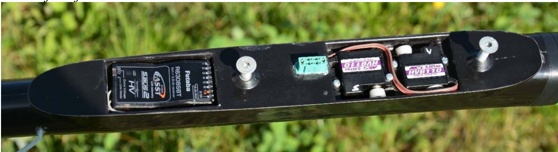
Servos and receiver installed in fuse
