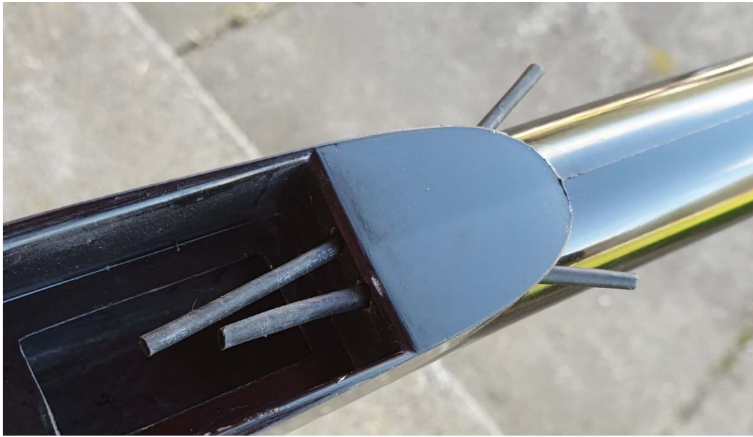
Antenna holes / guidance tubes
