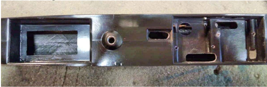
Cutting holes in fuse before assembly
