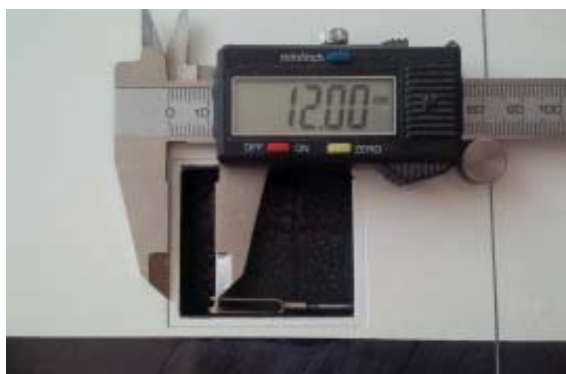
Pic. 7 Aileron control rod length
