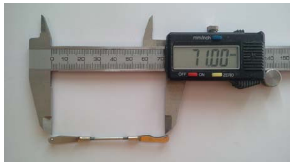
Pic.3 – Aileron push rods
