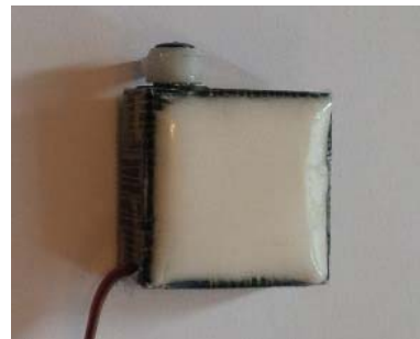
Pic.12 – Epoxy on servor
