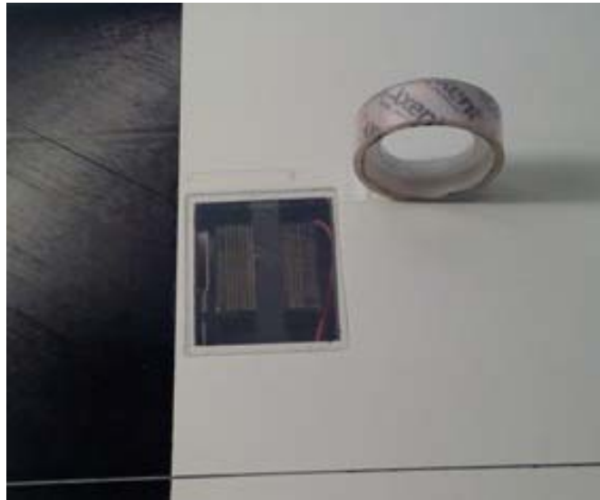
Pic.15 – Gluing flat servohatch Fix
