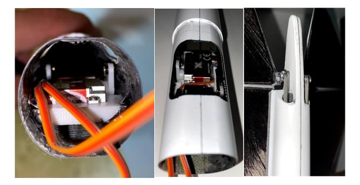
You see on the pictures below the tail servo mount. The linkage must be shorten tot he right lenght and grind. Be carefully that the Vtail pushrods have the right angle to go in the ruder hole.
