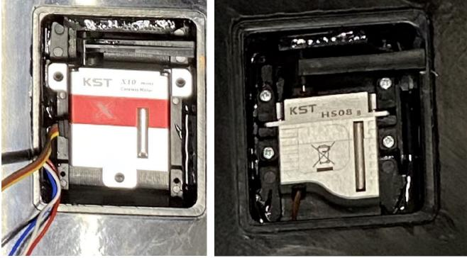
Glue the Servotrays in and make sure that it glued in well all arround. You have for wing Setup pattern teaching for Flap and Ailron. With the X10 and the second servo horn, you have ca 20% offset, with smaller servos more (40-55%)
